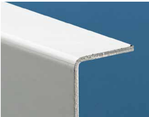
The comparison: Bending results with WingBend PLUS and standard-V-die
